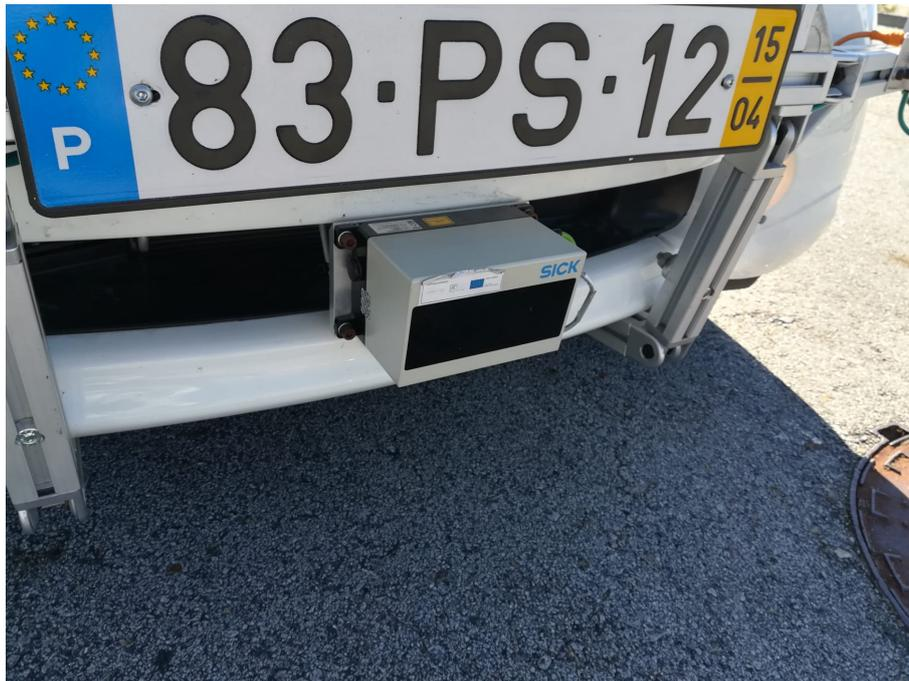
Figure 3.2: LIDAR placement in the *AtlasCar2*.
